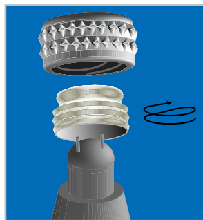
Cap Insert is threaded into the metal keeper with 2-pronged wrench.
